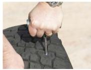
3. Insert the reamer into the puncture hole and push in whilst rotating the handle to clean out the hole. Reinflate tyre to help with insertion of cord.
