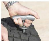
5. Firmly push the insertion tool and cord into the tyre until the sleeve is fully home against the tyre. A small amount of the cord should still be visible.
