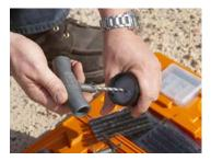
2. Apply lubricant to the spiral shaft of the reamer tool. This will help to probe the hole and temporarily separate the steel belts without damage.
