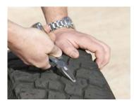
1. Remove debris from tyre tread or sidewall using a suitable tool such as a pair of pliers. Take care, as residual air will escape under pressure.
