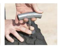
6. To remove the tool, hold the sleeve firmly against the tyre and pull up on the handle. Note: do not twist the handle. Trim the excess protruding cord with a suitable blade.
