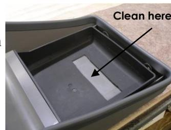
Peel one side of protective backing from foam strip supplied; apply pressure with palm of hand to adhere foam to exposed part of console. Peel backing off other side of foam strip and add one or more strips of foam to suit different size radios (see chart below). This will keep radio level with bottom of surround.
