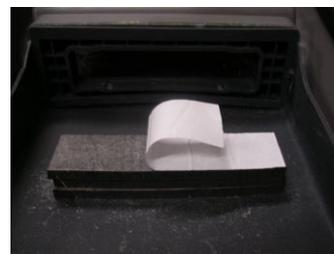
Insert radio on an angle until radio protrudes 15mm out over bottom of tray surround or insert and straighten; lay flat onto sticky back foam and apply firm pressure to top of radio with palm of hand for 30 seconds to ensure good adhesion.
