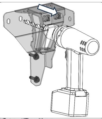
8. Using an Ø8.5mm drill bit, drill through the tub body at all four mounting slots. One is hidden from view (shown with the arrow) and accessed through the hole in the mount.
