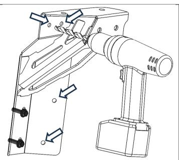
11. Using an Ø8.5mm drill bit, drill through the tub body at all four mounting holes.
