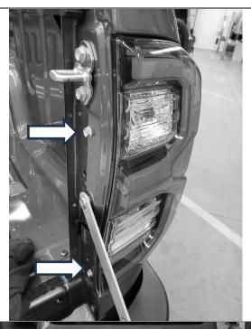
2. Remove both left and right taillights, unplug the lamps and place in a safe location.
