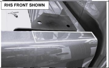
23. Cut two pieces of ABRASION RESISTANT TAPE 220 X 18 X 0.4MM to 160mm and fit to the front top surfaces of the tub as shown.
