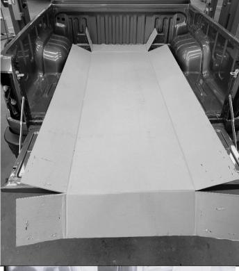
3. Remove the BED RACK carton lid, remove the large staples and place into the tub. The carton lid will protect the tub from scratches.
